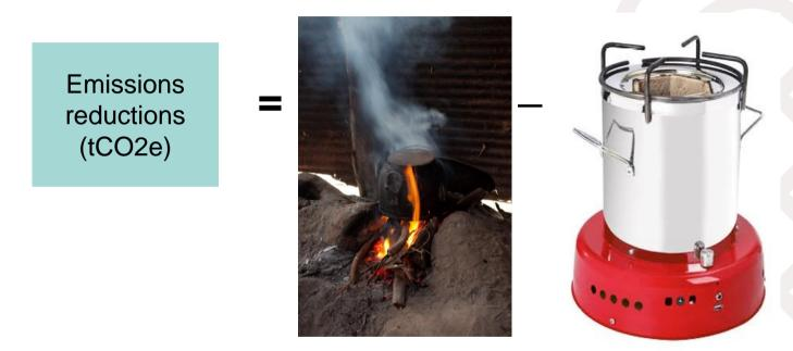
1 stove can reduce from 0.5 to 1 tonnes of CO2e per year
