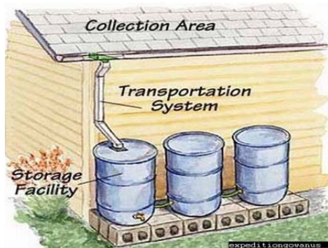
Example of a rainwater harvesting system
