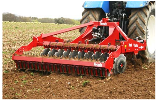
Disc harrow used for conservation tillage
