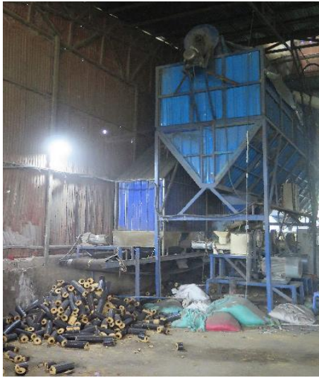
RICE HUSK BRIQUETTE PRODUCTION UNIT AT RANN SA RICE MILL
