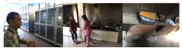
Chheng has designed and purchased drying equipment (left) powered by gas, as an improvement to the previous drying technique in frying pans (middle) powered by coal ovens (right)
