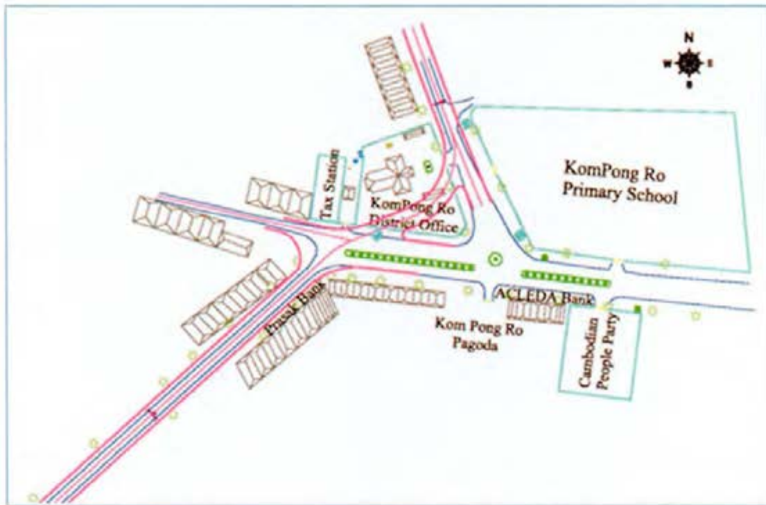
Figure 4 Realignment in Kampong Rou, PR314D
