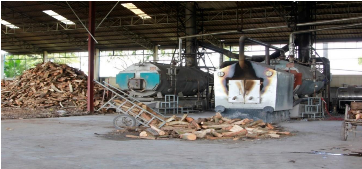
Figure 13. Many of Phnom Penh's factories are powered by charcoal and wood as fuel for boilers (photograph source: UNIDO)
